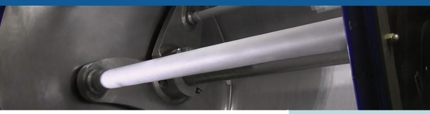
Shaffer's patented Refrigerated Agitator Assembly (U.S. Patent No. 9,295,956) design for single end drive mixers decreases dough temperatures by 3° to 5° F to stabilize and maintain your dough's ideal temperature by being in contact with the dough 100% of the time. The Refrigerated Agitator Assembly can be retrofitted into existing mixers to provide the most powerful cooling system in the baking industry.
