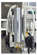
Stable sealing is achieved by adopting servo-driven film feeding roller built-in vertical seal unit.
