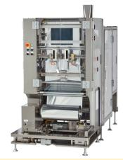
By installing a hem folding device (option), it is possible to make bag with Hem seal.
