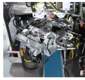
Servo-motor controlled End-sealing enables high-speed packaging, and a Seal-Contamination Detect Function is now standard feature.
