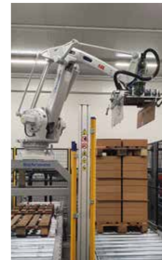
Robotic palletizer features a gripper head.
