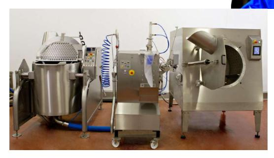
Basic cook-chill arrangement - Ready-2-Cook Kettle, Pump Fill Station, Tumble Chiller.
