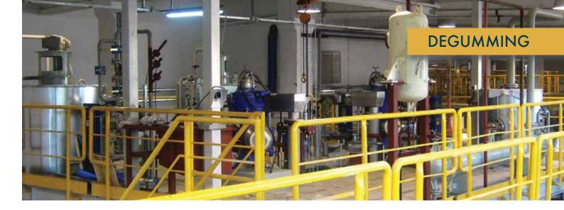
egumming removes phosphatides, commonly known as gums. Gums are either hydratable and non-hydratable phosphatides. Hydratable phosphatides are separated in the water degumming stage while non-hydratable phosphatides are removed by gum conditioning and alkali refining or enzymatic degumming.
