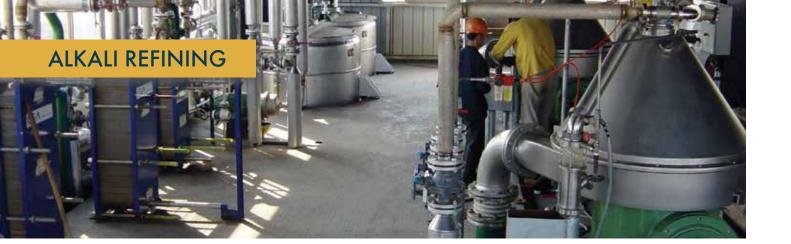
he process of neutralizing the free fatty acids in oils by a strong base (alkali) is known as alkali refining. The steps in alkali refining include gum conditioning, alkali neutralizing and washing.
