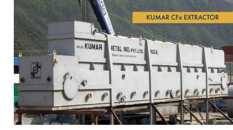
umar's CFx Extractor is of horizontal construction. It comprises an articulated band conveyor assembly which receives material from the feed hopper and transports it at a very slow predetermined speed from the feed to discharge end. The conveyor moves over rails suitably located within the extractor and rides on specially constructed sprockets at either end. It has an adjustable damper to regulate the height of the bed of material on the band conveyor.
