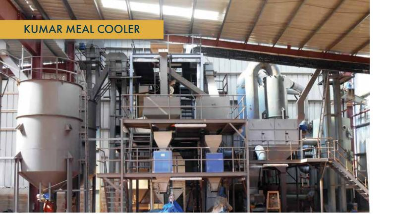
n applications where a separate cooler is needed, Kumar's vertical meal coolers reduce the temperature and moisture of the meal coming out of the Desolventizer Toaster.
