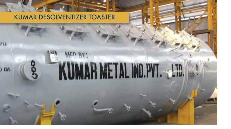
xtracted meal is transferred to the Desolventizer Toaster for removal of entrapped solvent. Desolventized material is conditioned by controlling and adjusting direct and indirect steam. Conditioned toasted meal is sent to meal cooling section for further processing.
