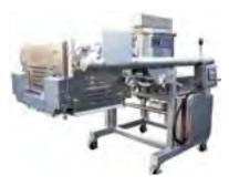
6 Piston Servo Filler with Bridge & Hopper Agitator
