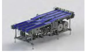
The ProLeaver CBI4 Cooked Bacon Interleaver is a modular paper dispensing system designed to accurately place the correct number of precooked foodservice bacon slices on paper prior to stacking. This system can run programmable paper length at speeds up to 60 sheets/minute/lane. Each lane runs independent of the others and all lanes can be equipped with a 2nd unwind to extend your run time.
