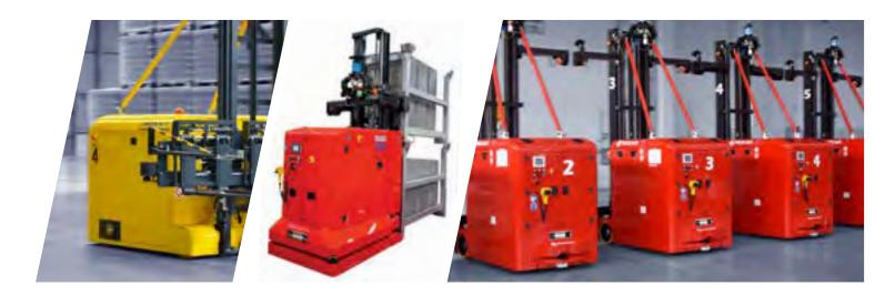
Proxaut AGVs can be divided into two major categories with unique options based on their applications. These can be highly customized or a standard model. All are powered by high performance, low maintenance lithium batteries.
