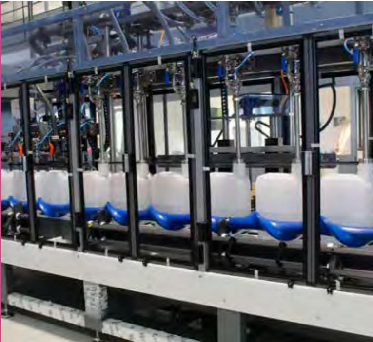
*Dosing of different products in the same filling cycle. The machine automatically mixes alkaline and acid products in the same filling cycle, avoiding pre-dosing mixing.*
