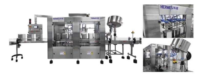
Thomason Automatic Monoblock Linear Weight Filling and Closing Machine model HERMES, with single lane conveyor, Four Filling Heads and one closing head.
