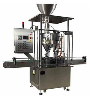
Thomason Automatic Monoblock Powder Filling and Capping Machines model ATHINA, are suitable to fill powder and granular products in Plastic-Glass-Metal bottles and jars, Cylindrical, Rectangular Shapes and close them with several options of Capping Heads, according to the cap type.
