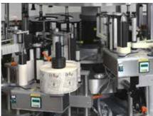
Thomason Rotary Labelling Self-Adhesive Machine NEFELI-AD, is a Multi-Labelling suitable for the application of labels on Cylindrical, Conical, Square based, Oval and Rectangular containers.
