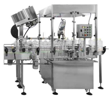
Thomason Automatic Capping Machine, model PEGASUS/D8 with mechanical indexing movement of the star-wheel controlled by inverter for rotation speed adjustment and smooth operation and with one Capping Head suitable to handle all types of caps.
