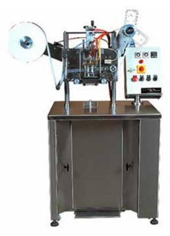
Thomason Semi-Automatic Foil, Aluminium or Plastic, Cutting and Sealing Machine model ARIA/1-S. Manual loading and unloading of the bottles/jars.
