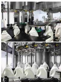
This Monoblock is based on a Volumetric (Piston) Filling System with the typical advantage and flexibility to fill many kinds of products with Low to High Viscosity.
