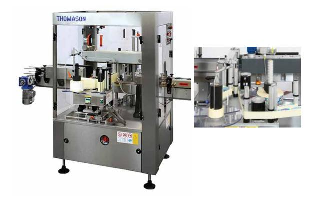
Thomason Linear Labelling Self-Adhesive Machine LEDA-AD, is suitable for the application of labels front and back on Flat - Oval - Square - Rectangular bottles and Partial or Wrap-Around label on Cylindrical containers.
