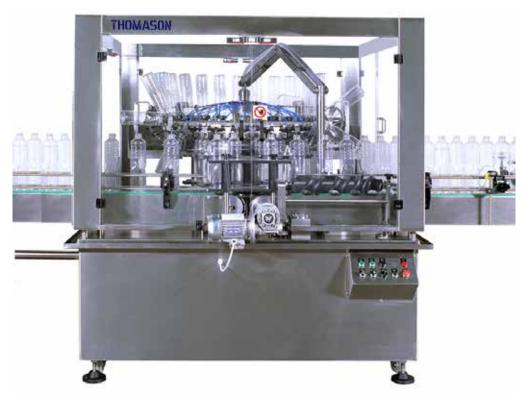
Thomason Automatic Rotary Water or Air Rinsing Machine model KALIPSO suitable for Rinsing Plastic - PET - Glass - Metal bottles and jars of different shapes and sizes.
