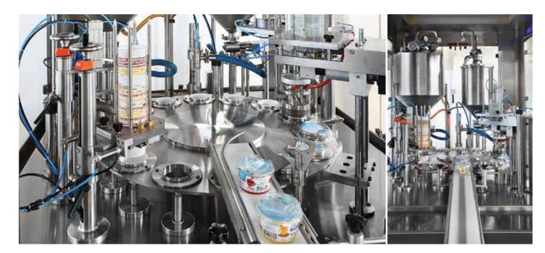
All functions are fully automatic and equipped with highly flexible mechanics. This machine can be offered with One to Four pockets depending on the cups size and the speed requirements.
