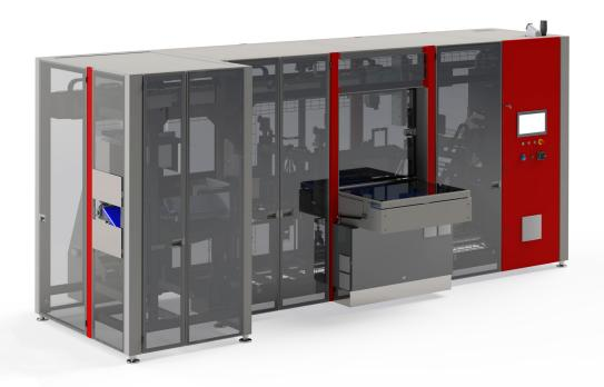
The Aligning Collating Multipackaging machine, or ACM, is designed to process pre-packed individual product portions directly from a Vertical Form Fill machine (or VFF). The ACM is a fully automated multipackaging machine, used for packaging into pre-made, wicketed polybags.
