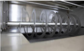
Helical spreader ensures level product bed
