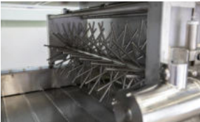
Adjustable spike roller gently separates coated products
