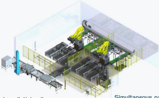
Complete palletizing line with wrapping machine suitable for 30 pallets per hour
