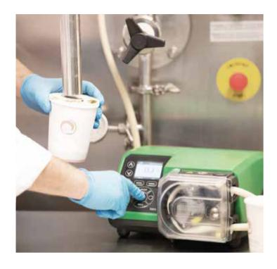
Peristaltic pumps can handle aggressive and shear sensitive fluids. The pumped fluid is totally contained within the tube, providing complete isolation of the fluid and no cross contamination.
