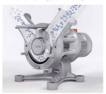
draw in more fluid, resulting in a smooth flow with virtually no pulsation. A gate stops fluid flow from the higher pressure outlet to the low pressure inlet.
