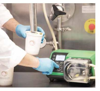
Peristaltic pumps can handle aggressive and shear sensitive fluids. The pumped fluid is totally contained within the tube, providing complete isolation of the fluid and no cross contamination.
