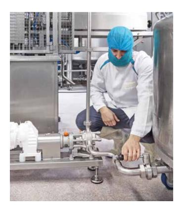
Certa by MasoSine outperforms lobe pumps in critical food and beverage applications. The sinusoidal rotor design of our MasoSine pumps delivers a lower shear, gentle pumping action that safely transfers delicate food products without risk of degradation.
