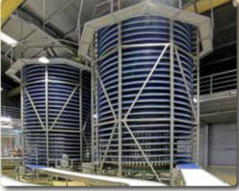
SARCOOL Series - Spiral Cooling Towers Intralox DirectDrive™ Technology
