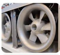
High-performance fans can be adjusted for each freezing zone, reducing power consumption and optimizing airflow for each product type.
