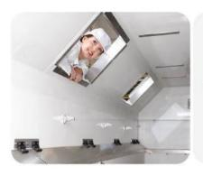
Hygienic design with rounded corners, no joints, and sloping surfaces for easy drainage and efficient cleaning.
