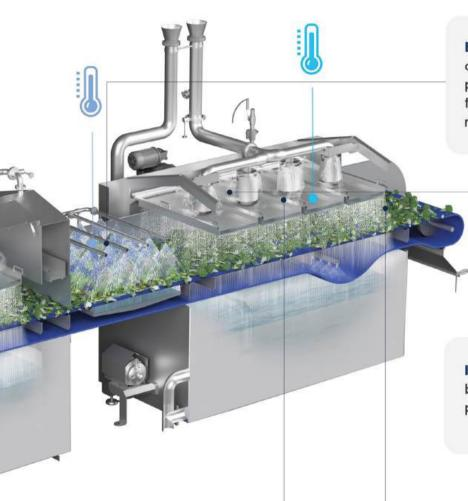
Efficient heat-recovery section uses ambient temperature water to lower the product temperature. The water that flows over the hot product is recirculated, requiring minimal energy for reheating.
