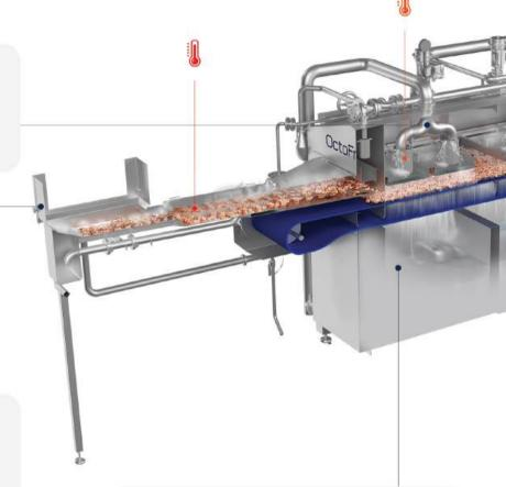
Weighing belt option allows for precise feeding into the cooker. For maximum flexibility, the OctoFrost IF Cooker offers three infeed options: bulk, belt, and tray infeed. Additionally, a "finger-lay" infeed belt can be attached as an alternative to tray feeding for curl control.
