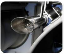
The foam generator, combined with the fans, distributes detergent inside the freezer for an efficient cleaning cycle. Few moving parts result in minimal maintenance needs and ensure a reliable freezer.
