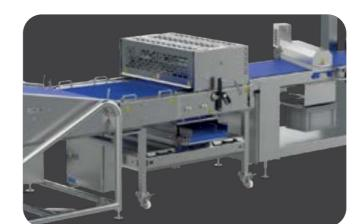
Do your customers want tasty donuts that are crisp, wellshaped and have a good texture? With the Smart Donut Line, you have a machine that can offer exactly that. The donut dough is rolled out into a stress-free dough band and the donuts are then stamped out of it.
