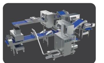
With the MLC 4.0 Block Line, dough blocks with 2 to 400 fat layers can be produced, depending on the selected layout. A dough band is automatically shaped, with the option of folding in fat, then rolled out and the band is cut into pieces.
