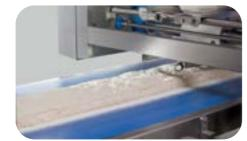
Many RONDO lines are modular in design, allowing you to automate any or all of the work steps. We supplement our feeding lines with our various dough band formers and fat pumps, for instance. The innovative MIDOS dough band former was developed in an ASTec design and works without process flour and oil.
