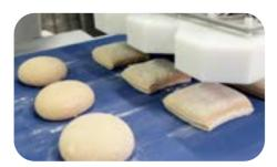
Numerous modules, such as dusters and moulding units, round out your bread line. The innovative RONDObot simulates manual round moulding and forms identical round and oval breads and rolls of excellent quality.
