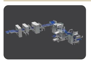
The MLC 4.0 laminating line automatically produces uniform, laminated dough bands. and continuously feeds them into your make-up line. With various layouts and accessories, the right solution can be found for every requirement.
