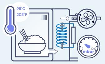
2 The vacuum pump starts and reduces the air pressure in the room from 1000 mbar to the desired pressure.
