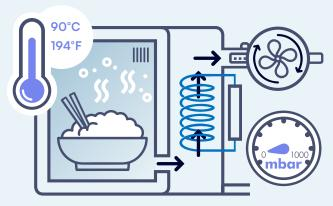
3 A small amount of water within the product will start boiling when pressure reaches temperature level of the product. This boiling process requires heat that is extracted from the product, enabling the cooling.
