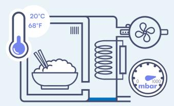
5 The cycle ends when the product is cold and the pressure returns to 1000 mbar.
