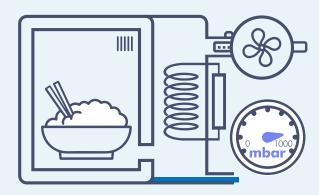
The condensed water is drained and the vacuum cooler is ready for the next load.
