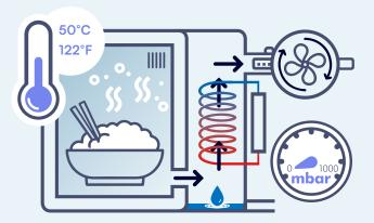
4 The water vapor is condensed by passing a "cold wall". The dried air goes out through the vacuum pump.
