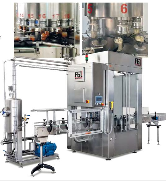
Once the filling phase is completed, the closing systems come into action to complete the packaging of the containers.
