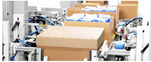
Lidding Machines are automatic modules designed specifically for sealing lids onto cartons. Using single or multiple lidding heads for a flawless lid placement for all your secondary packages.
