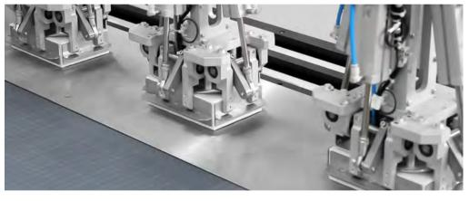
GPI's Closing Machines are automated modules designed specifically for sealing flaps carton, featuring one or more application heads for optimal performance, maximizing your production line's output.
