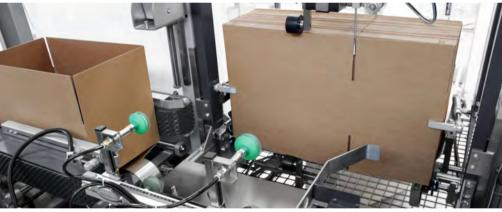
Case Erector for RSC case (regular slotted container) are automatic machines engineered to shape and securely seal the bottom flaps of the case using hot melt glue or adhesive tape.
