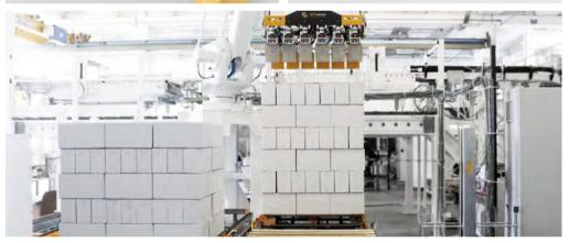
GPI Group produces robotic palletizers capable of handling multiple infeed and outfeed lines, offering extensive plant customization options. Solution that stands as the optimal choice for boosting productivity
