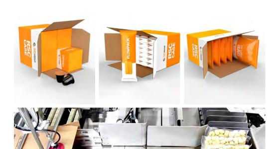
GPI's Side Loading Unit for RSC cases are automated system for the lateral infeed products, by pushing them into the case. It's a practical solution ideal for cartoning various products with high speed and fluency.
