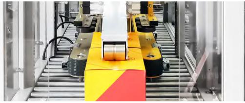
Case Sealer for RSC case are automatic machines for upper flaps sealing using hot melt glue or adhesive tape. These machines are compact and easy to adjust, for an effortless integration into all packaging processes.
