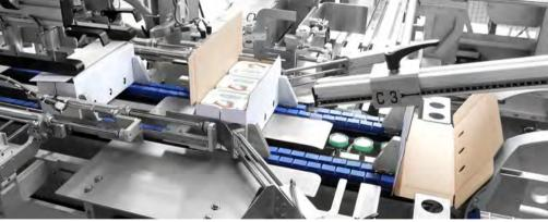
Wrap-around case packer provide a versatile and efficient solution.
