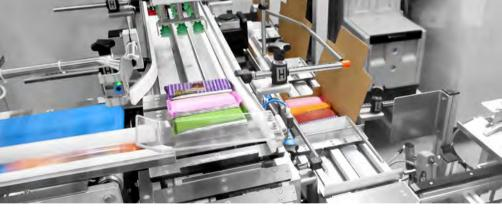
All in One Units for flaps carton integrate forming, packing, and closing phases into a compact and highly functional design with great attention to the accessibility for maintenance activities.
