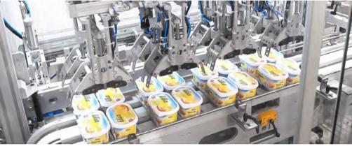
All in One Units for RSC Case are a combination of forming, packing and closing phases merged into a unique and functional design with minimum footprint and high reliability.
