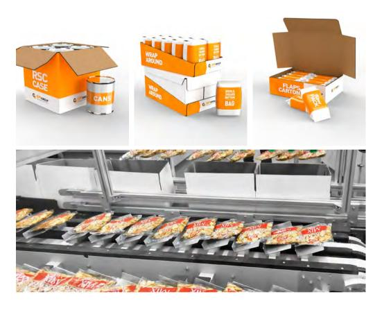
Top Loading Units are very productive packaging solution, engineered with an advanced 2-axis robotic system for packing products into all secondary packaging, ensuring flexibility and efficiency.
