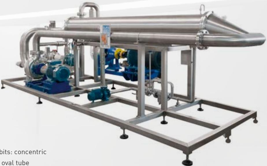
Special attention is paid to diced fruit and tidbits: concentric tube heat exchangers can be replaced by the oval tube version, which allows working pressures to be reduced with a consequent improvement in the quality of the output product.
