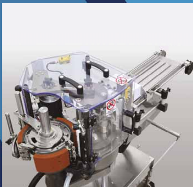
MAK-GS cold glue labelling station
