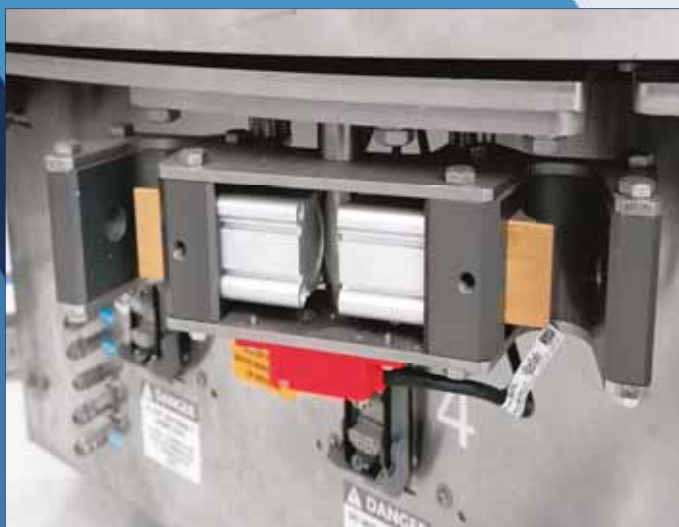
PNEUMATIC connection of removable modules (Optional)
