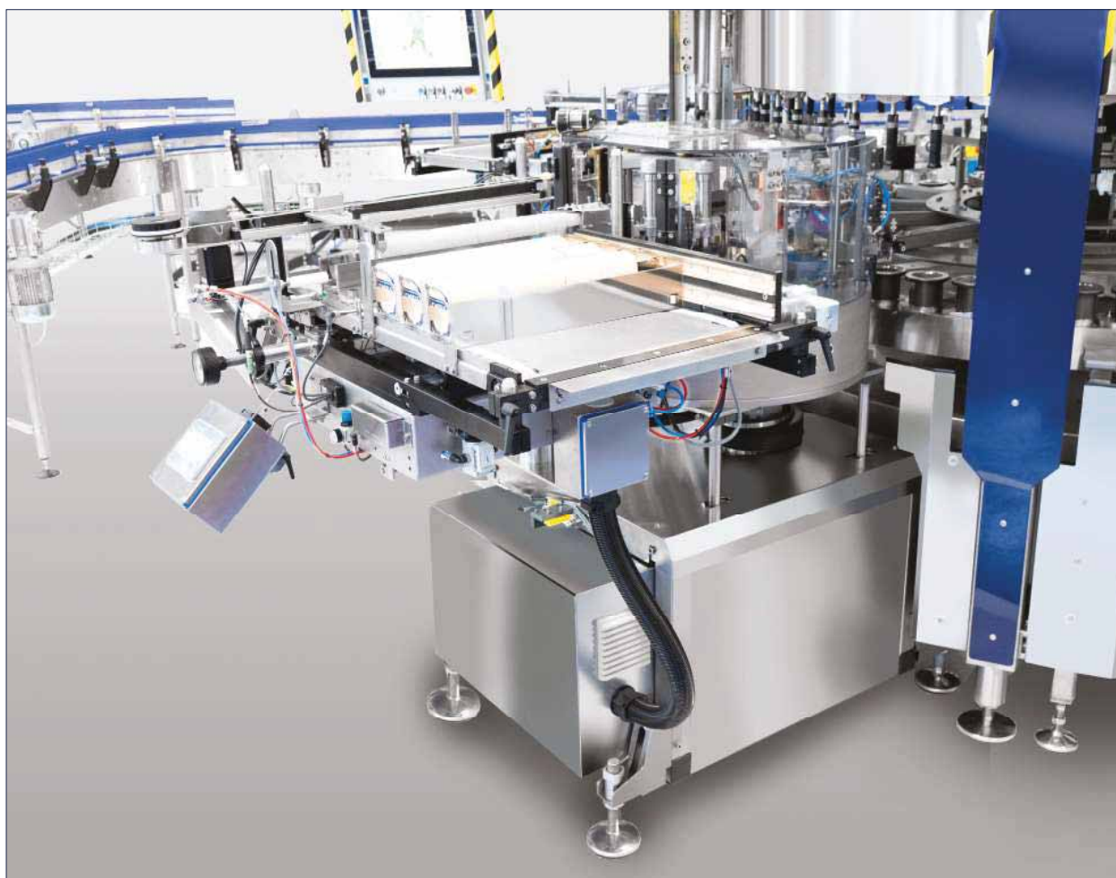
MAK-GHS station with automatic label magazine
