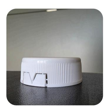
Apart from the edible oil segment, we are proud to serve India's dairy industry by manufacturing 38 mm HDPE caps for flavored milk bottles. These caps can be customized to meet specific client requirements. We also offer a variant with a notch, designed to make the induction wad easier to tear for enhanced user convenience.
