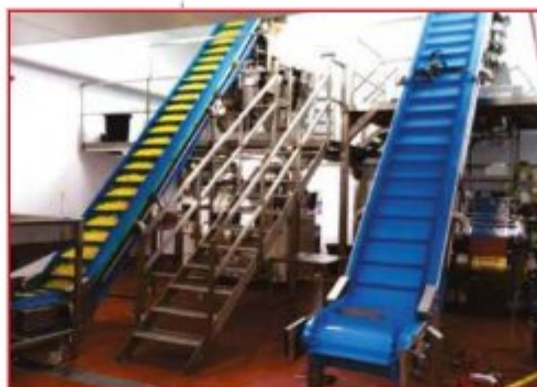
FDA Certified Thermodrive Sidewall GooseNeck Conveyor for Process Line
