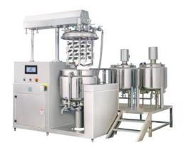
Prism has been designed & manufacturing fully automatic Semi solid manufacturing Plants are ideal tools for the pharmaceutical & cosmetic industries for the production of Ointment, Cream, Lotion, Gel, Tooth Paste & emulsions & homogenization. Available model 50 Liter to 5000 Liter working Capacity.
