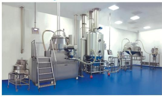
Prism Integrated granulation lines as per current Good Manufacturing Practices requirements that product is fully contained during processing to protect operators and environment. Also improved productivity through closed materials transfer, automation, increased yields and efficient cleaning procedures.
