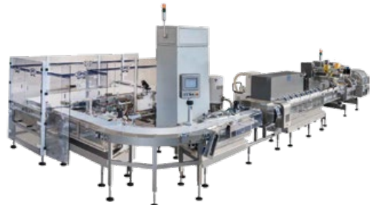
High speed automatic packaging lines for enrobbed sponge cakes
