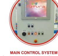
Our main computer allows for control of various grading parameters throughout the entire line, including weight, diameter, colour and external quality.
