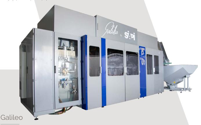
After an intense R&D activity, SIAPI introduces in the market the revolutionary technology of progressive preform feeding: an innovative solution with fixed molds and preforms rotary movement.
