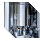
Rotary can seamers, food or beverage version available, featuring 2 to 6 heads, up to 600 cpm. Suitable for diameters from 52 to 99 mm.
