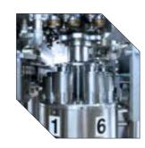
Rotary Can seamers, food or beverage version available, featuring 4 to 6 heads, up to 600 cpm. Suitable for diameters. 52 to 105 mm.
