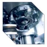
Stationary can seamers for food products, ideal for diced tomatoes and fruit salads; 3 and 4 seaming head models, up to 200 cpm. Suitable for diameters from 99 to 180 mm.
