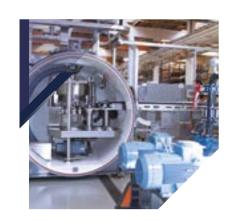
INDEPENDENT VACUUM PUMP UNIT, EQUIPPED WITH 2 PUMPS AND COOLING TANK WATER RECYCLING.
