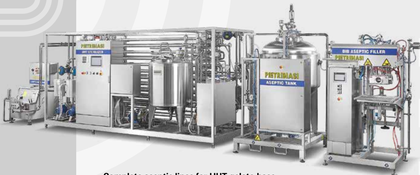
Complete aseptic lines for UHT gelato base
