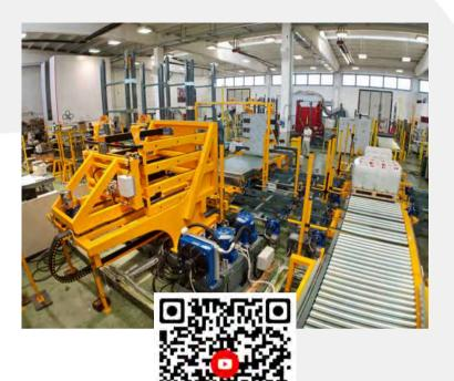
Side Pusher Logy is one of the fastest no titlting pallet exchange solutions, capable of handling up to 120 pallets per hour at maximum capacity.
