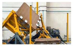
This option maintains the slip sheet with the load during the pallet change cylce
