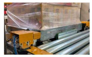
This station cuts the wrap on the load, reducing work risks and improving efficiency.
