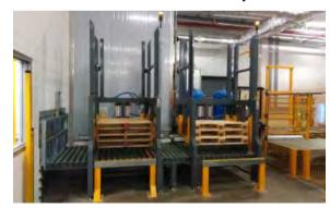
Capable of stacking various pallet types ready to be used.
