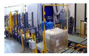
It's a system capable of load shape detection in order to control it before entering inside the machine.
