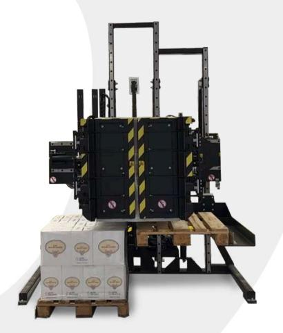
*Pantera* is the ultimate version of layer picker solutions that efficiently lifts, splits, and laterally transfers the load onto a new pallet in the safest and fastest manner.
