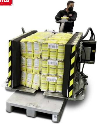
Falcon Wings is an electric-powered mobile pallet changer machine that securely locks and lifts the product from the pallet.
