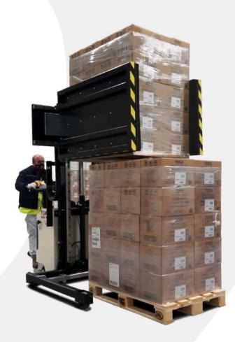
Side Press Splitter is a portable layer picker capable of both splitting product-stacks up to 1.400 mm and exchanging pallets.
