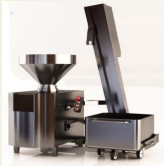
For Lifting & Tilting of Buggies in Vacuum Filler Machine
