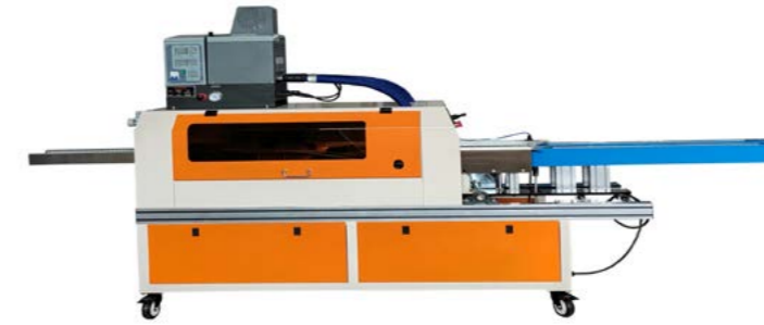
Smart box packer BP010.. Wheel rolling glue or equipped with glue spraying machine. Easy for changeover
