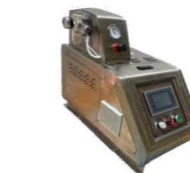
Hot-melt adhesive machine HMA010, 8L glue tank, PLC control, Stainless steel body/ food safe; Piston or gear pump
