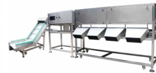
Weight sorting and grading machine
