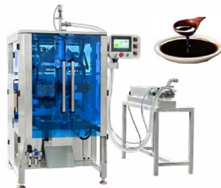
Liquid pump and meter + VFFS
