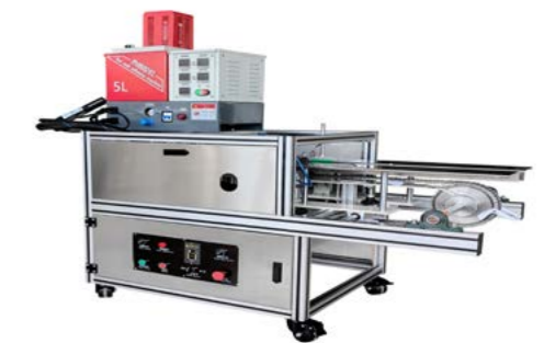
Smart box packer BP040. Automatic changeover, equipped with glue spraying machine
