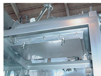
◆洗浄時（底蓋閉） At Circulation Washing (Bottom lid close)
