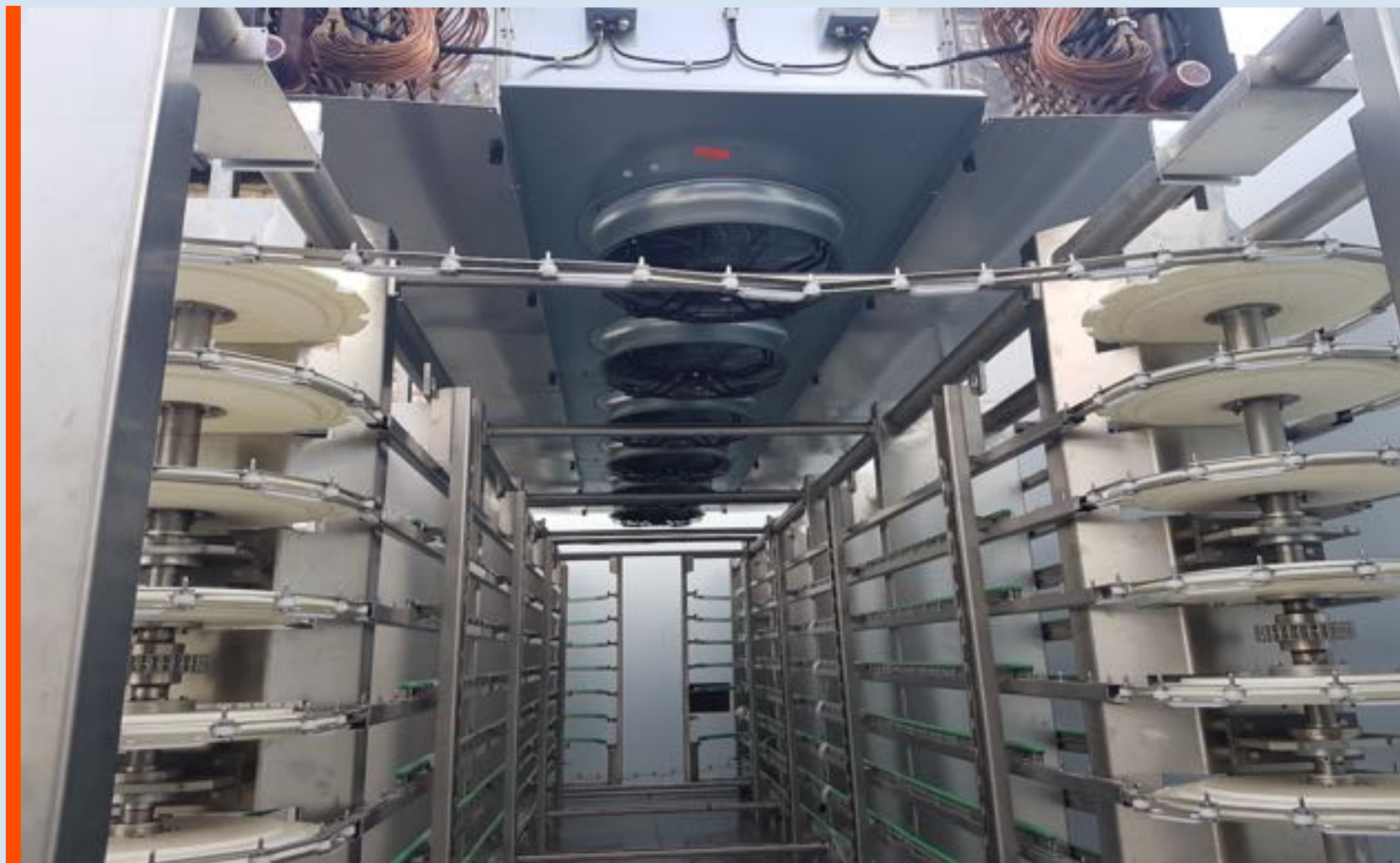
Inner view oft the tunnel with trays and extruded product on stick
