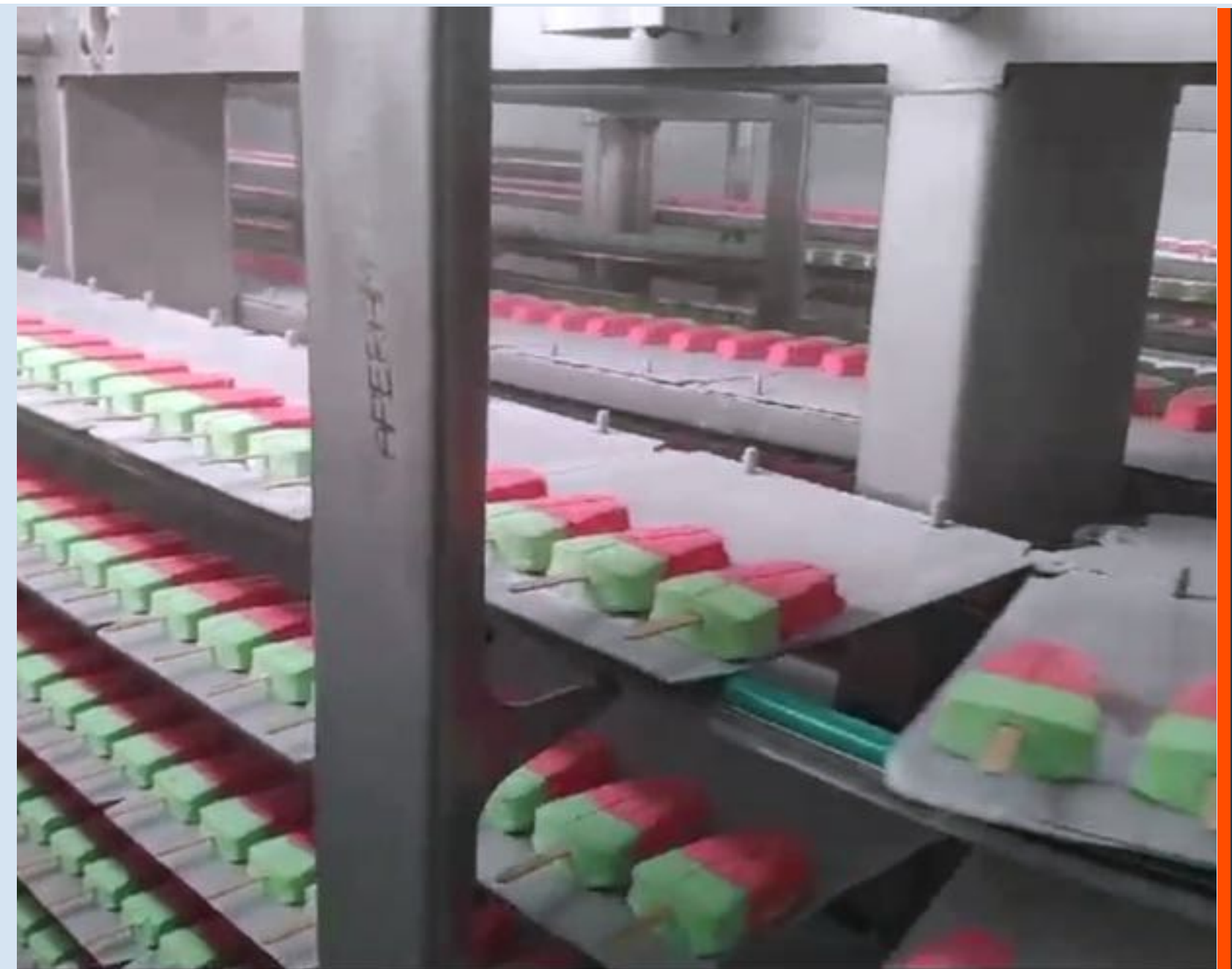
Inner view oft the tunnel with trays and extruded product on stick
