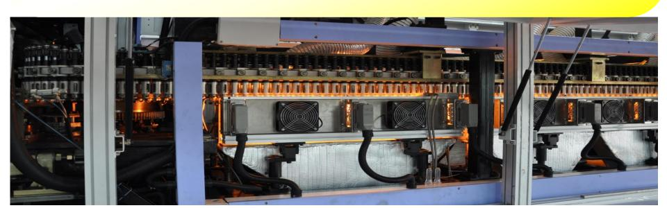
Adopt the merits of heating oven from oversea companies, new design of building block heating oven, install the special lengthen short wave infrared heating lamp, for the further optimization of filament wave length spectrum and reflect coating, the reflection efficiency is greatly improved, heating oven more energy saving, installation and maintenance more convenient;
