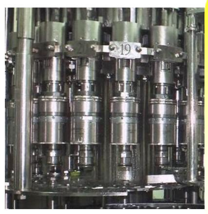
Adopt capping head of magnetic constant torque, the capping effect stable and reliable, defective rate ≤0.2%;
