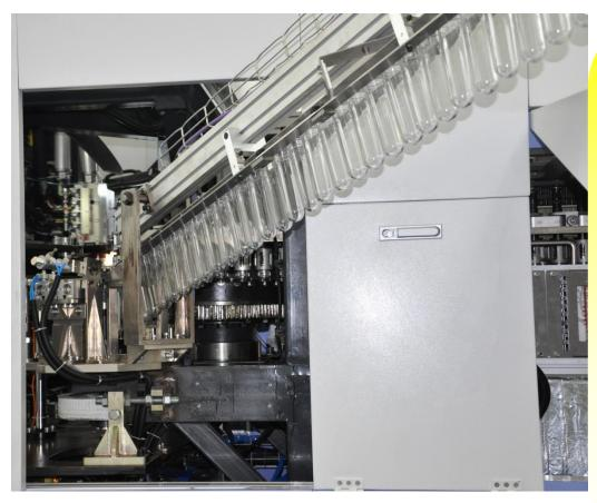
**International matured and stable** method of perform supply and unscrambler, perform enter into elevator from hopper, the perform transit to unscrambler by elevator, 2 incline rotating rollers automatically arranging the dropped performs and output it from unscrambler orderly, the surplus performs will back to hopper by reject wheel and return through backflow tunnel. Fully automatic control for arranging performs, high efficient but do not hurt the preform's surface.
