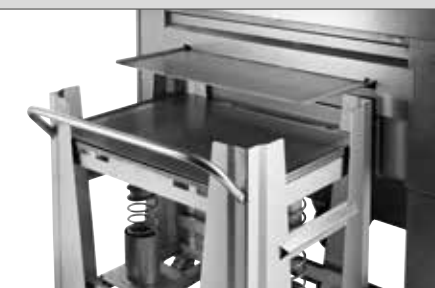
After the cleaning process, the trays drop into the tray wagon. When the system stops, the tray wagon containing the clean trays is removed, and an empty wagon can be put into place. The system is now ready to continue cleaning more trays.
