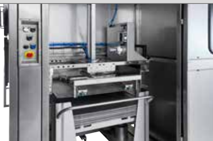
A pneumatic-operated vacuum system lifts the tray from the tray wagon into the tray cleaner system.
