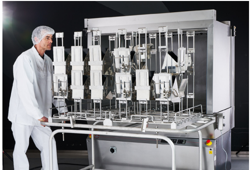
The trolley with the scales components safely fixed is rolled to the front of the JEROS ACE system.
