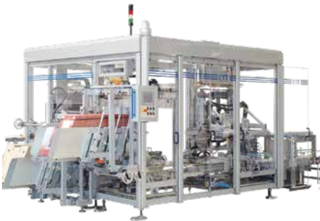
Compact system for producing two-piece cases.
