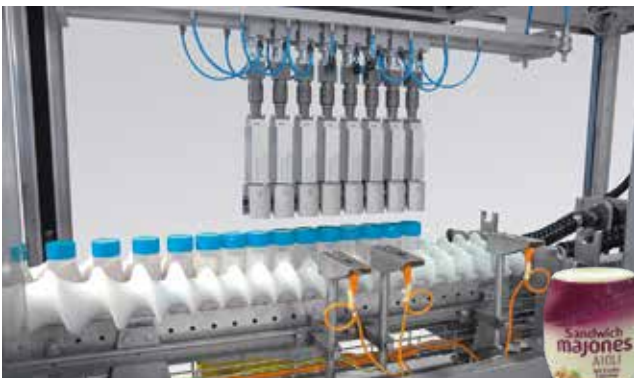
Integrated packing module with collating scroll.
