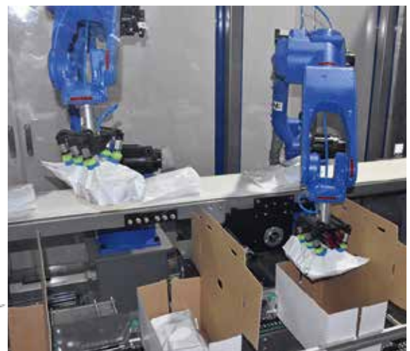
6-axis robot with line tracking for pouches.
