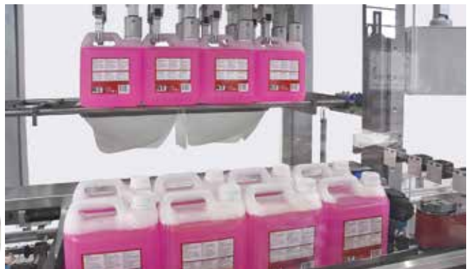
Packing of canisters with layer grouping device.
