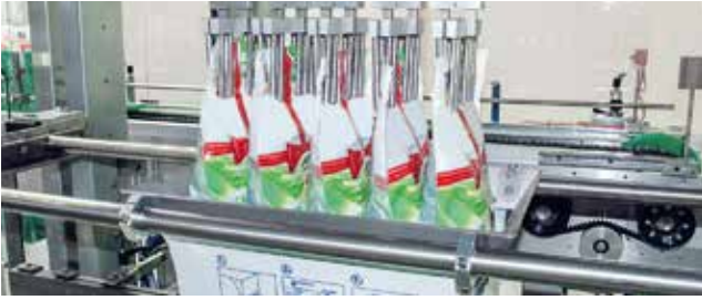
Packing of bags with multistep collating unit.
