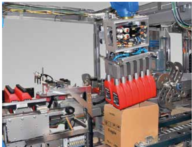
Robot loading products into the cases.
