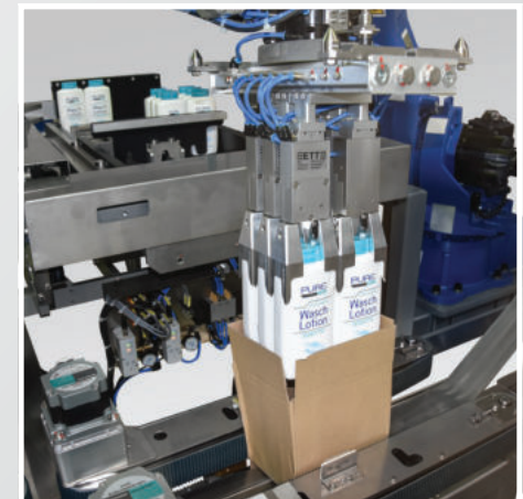
Full collation insertion of the products by robot no. 2
