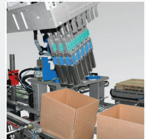
Dynamic insertion of a complete layer of products into the case
