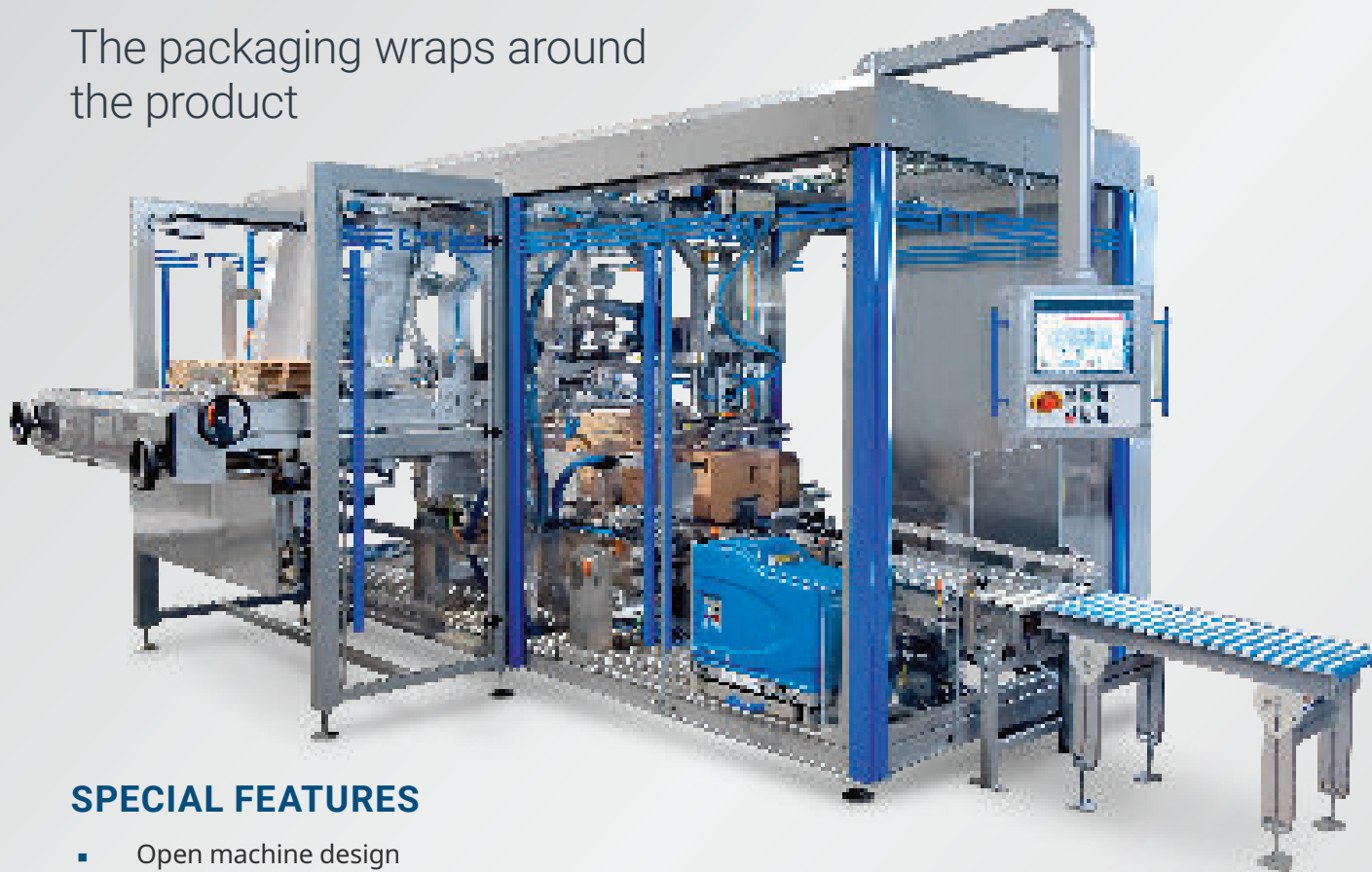
Product collation (cans) for trays with full wrap; multilayer packaging also possible as an option
