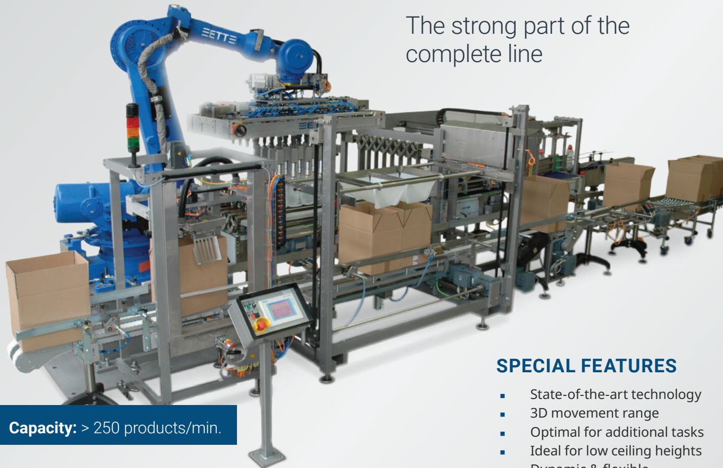
Scroll collation with rotation and insertion in rows
