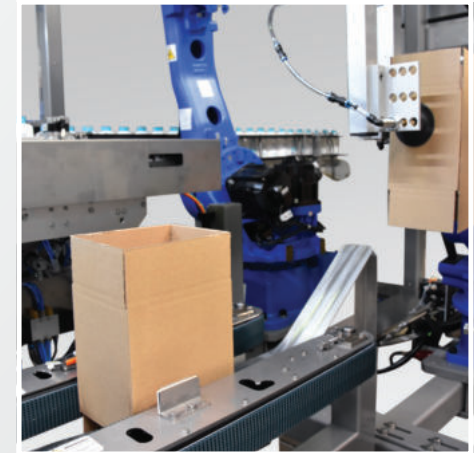
Blank removal and subsequent unfolding by robot no. 1
