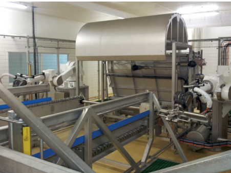
Robotized bag discharge system
