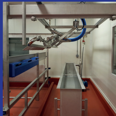
COP tank for the multitubular distributor
