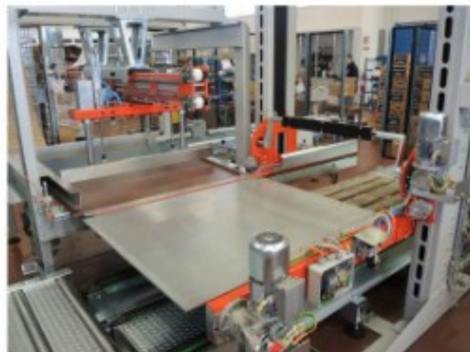
UNI601 1,5 layers/minute Semiautomatic machine with low-level infeed
