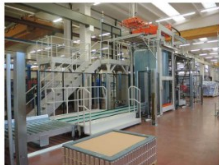
UNI550 4 layers/minute Automatic machine with sweep-off system and high-level discharge
