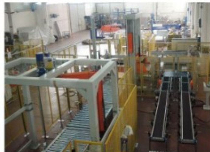
UNI600DI 4 layers/minute Automatic machine with low-level double infeed
