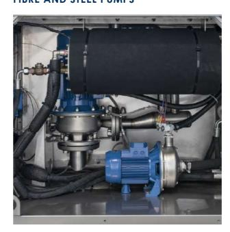
To ensure maximum cycle quality, the LCF 1500 3P is equipped with two 2.6 kW fibre pumps operating at full power. The heavy-duty 4k models feature two 4kW stainless steel pumps, the most powerful in their category.
