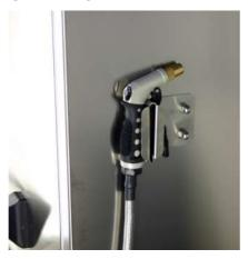
It allows the machine to be cleaned at the end of the day and the material to be pre-washed before the cycle starts.
