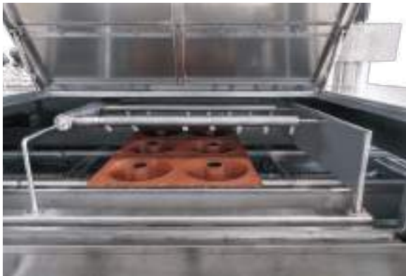
Demountable fixed washing sprays with quick connection bayonet coupling.
