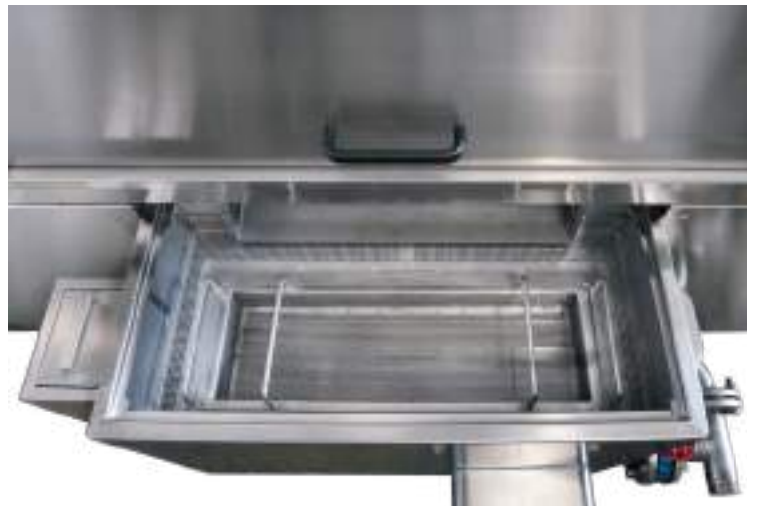
Double external filters for washing tanks.
