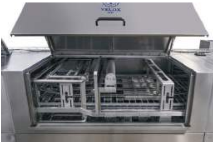
Demountable rinsing zone with micro economizer. It allows water to flow only in the presence of trays to rinse.
