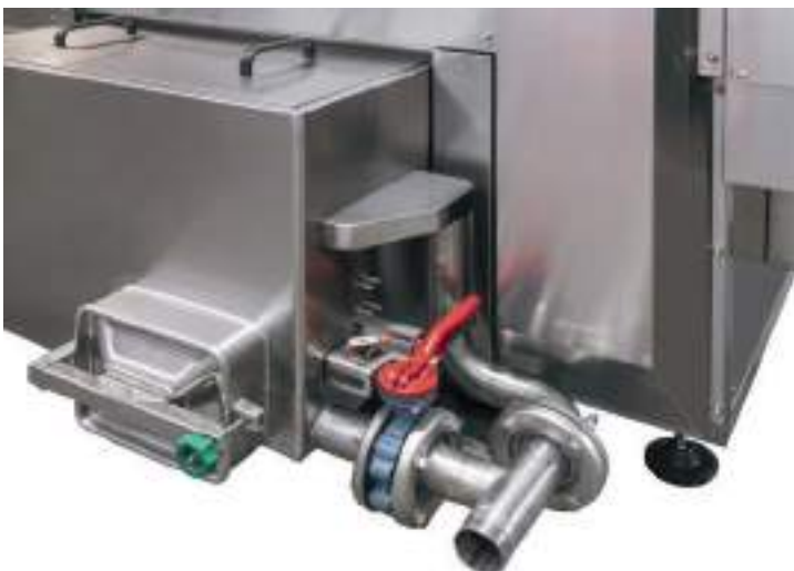
Drain with safety micro to prevent water leakages.
