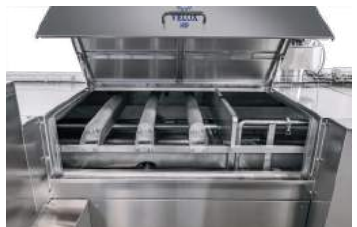
Drying with upper and lower air blades with adjustable inclination.
