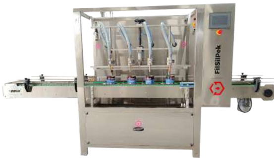
Automatic Multi Head Load Cell Base Filling Machine
