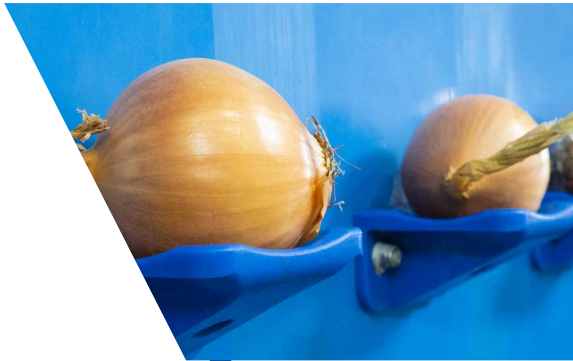
Infeed belt with special cups, producing a 99-100% fill rate
