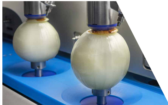
Unique upper and lower coring system, increasing yield by up to 10%
